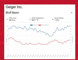
For each tank, ranchers can view the water level and water temperature. The graph provides a visualization of device readings.
