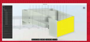
ZeroDelta's viewer highlighting a wall where no points were detected.
